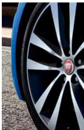
19" 5-Split Spoke 'Style 5031' Silver & Diamond Turned Finish O29UR Banden vóór / achter: 225/40 R19 97Y / 255/35 R19 97Y zomerbanden
